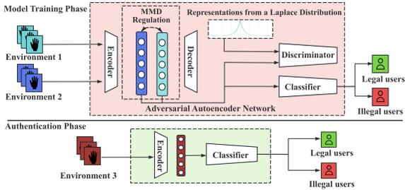
Fig. 7. The cross-environment adaptation module with user classifier.
